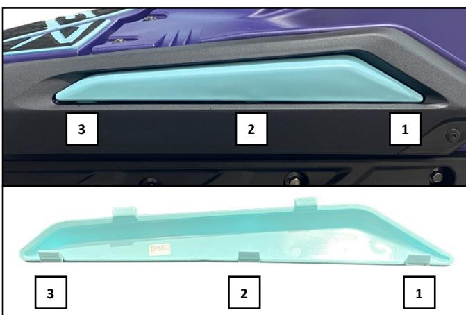
Start by prying up at forward locking tab [1]. Then, move middle tab [2] and finally rear tab [3]. Rotate bottom edge outward to remove insert. **NOTE: Do not pry at top or attempt to remove top first.**
