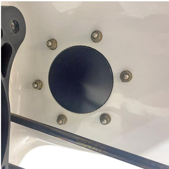
On right side of transom, **warm** boarding step bracket using a variable temperature heat gun or hair dryer to loosen adhesive backing. Carefully remove bracket and set aside for later.
