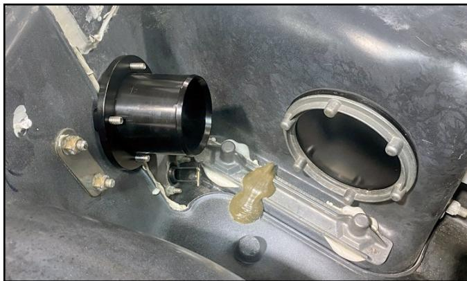
Modify boarding step bracket previously removed by removing 3/8" from lower boss.
