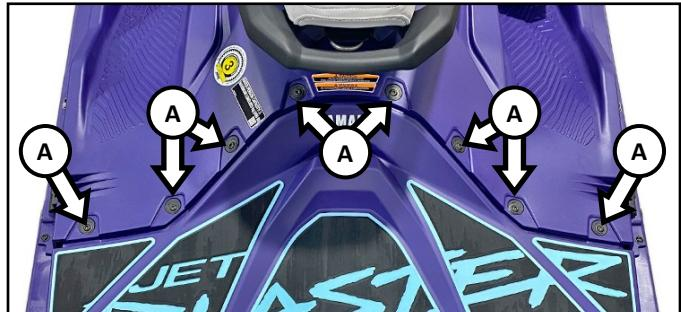
Replace rear bumper. **NOTE:** Reconnect reverse cable at reverse bucket (left side).
