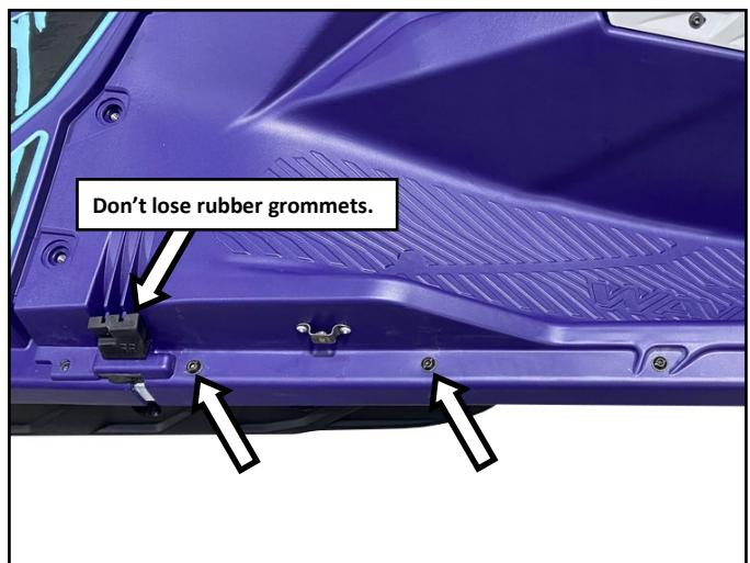
While raising rearmost edges of center deck section, remove rear deck section completely and set aside.
