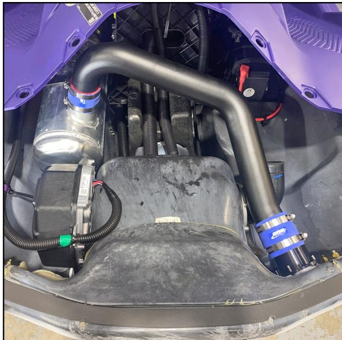
Verify alignment of exhaust tube and tighten clamps (4). **NOTE: Do not overtighten clamps.**
