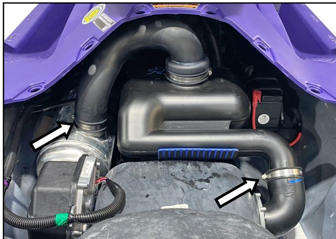
Remove exhaust baffle assembly and discard.
